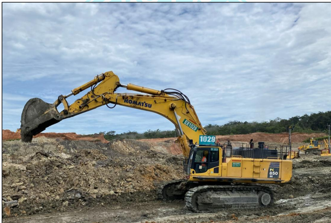
Gambar C.1 Alat Gali Muat Excavator Komatsu PC 850
