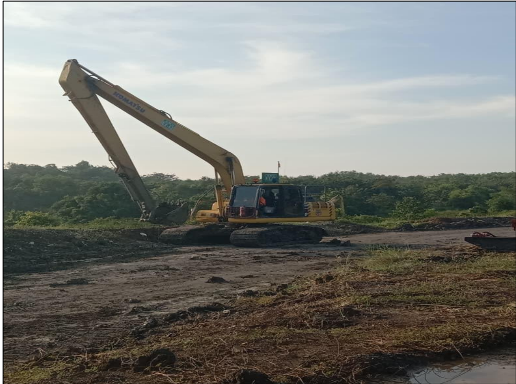
Gambar E.3 Excavator Komatsu PC210 Long Arm
