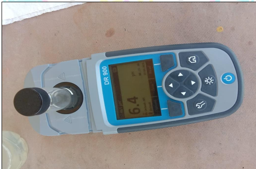
Gambar E.10 Alat Pengukur HACH DR 900 Portable Colorimeter
