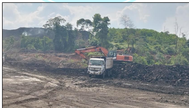
Gambar 2.2 Metode strip mine mining
