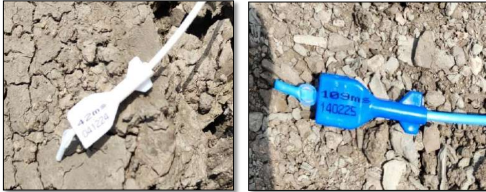
Gambar 3.21 (a) Surface Delay 42 ms dan (b) Surface Delay 109 ms
