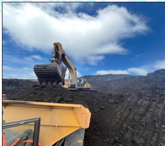
Gambar I.2 Proses Loading Batubara ke ADT
