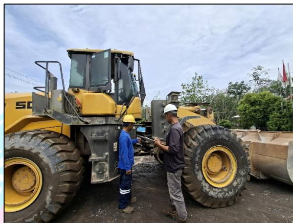
Gambar 4.1 Kegiatan P2H Wheel Loader SDLG L956F
